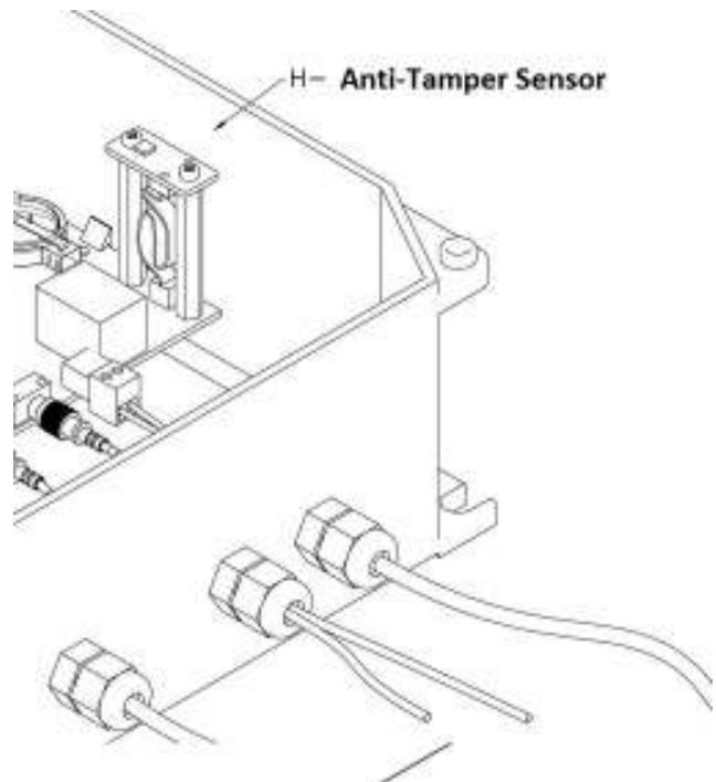
**11) 4-** Connect the alarm relay (10A to 240VAC) to the alarm system; you can place the anti-tampering sensor in-series.
