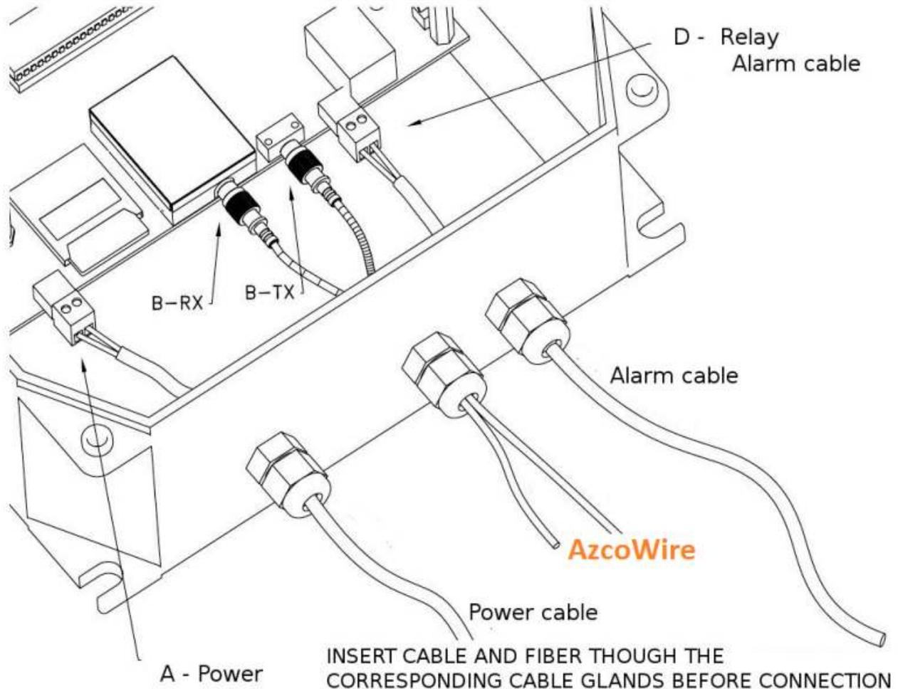
**8)** Connect the terminated AzcoWire to the *LightFence* controller.
